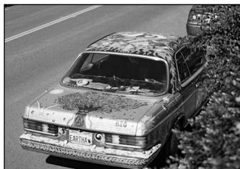
*This diesel Mercedes has been converted to burn veggie oil, diesel or biodiesel. Cost - \$5,000 and up + \$2,500 conversion to burn veggie oil costing \$1 per gal and up - 30mpg.*
